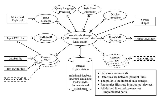
This data flow diagram provides an overview of the architecture of the workbench. The central processing is performed by the Workbench Manager which works on one or more XML files converted to the internal representation format plus one or more style sheets. On the basis of these files and through interaction with different processors it is able to perform the tasks described in the abstract above. Arrows indicate the main lines of the communication flow.
